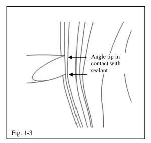
**If the vehicle has a sealant issue:** To push back sealant, align the adjustment tool to the edge of the door, with the angle edge positioned toward the inside of the door (Fig. 1-3).
